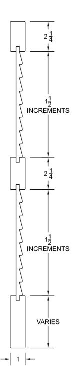
Millennium Wood Composite Faux Louver shutters are built using dowel construction. They feature eased edge stiles and rails and "flush face" design (all stiles and rails are the same thickness). Millennium shutters are primed with an option for prefinishing with either standard or custom colors.
